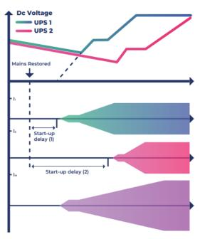
Dc voltage and AC current behaviour using different value for delay time
